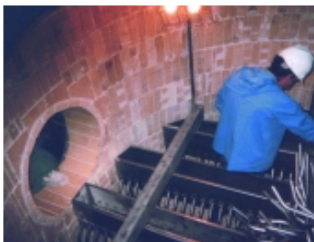
The Koch distributor is designed in a manner that completely covers the cross section of the tower and results in better absorption.
